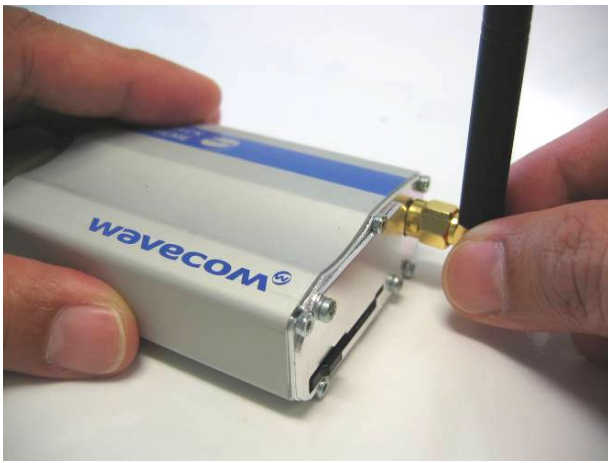
Attach the GSM antenna
