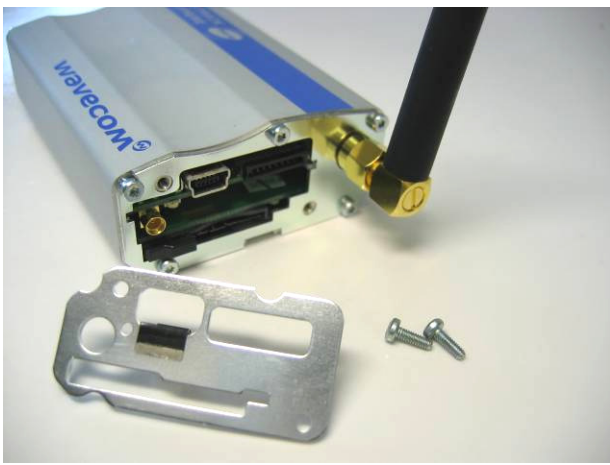
Place the supplied new backplate
