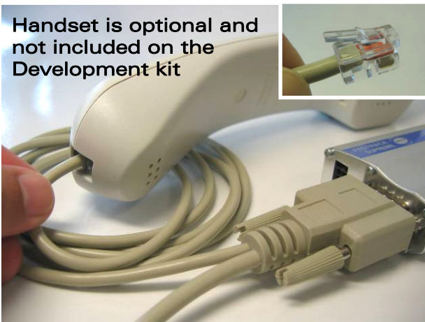
If handset is available connect the 4P4C standard handset cable to the handset
