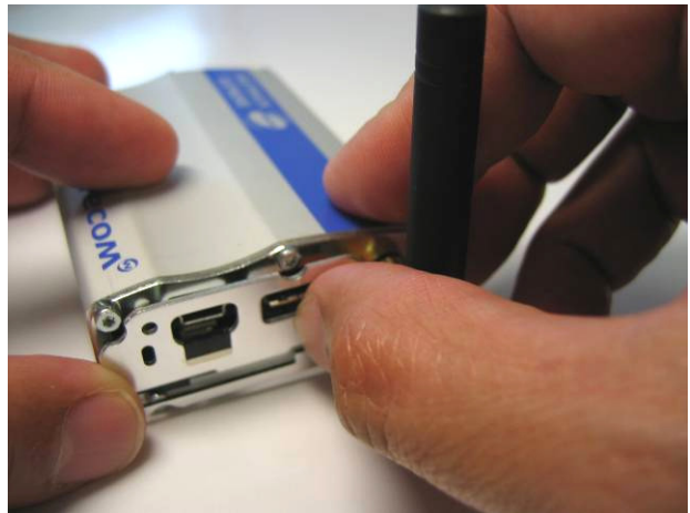
Align the new backplate
