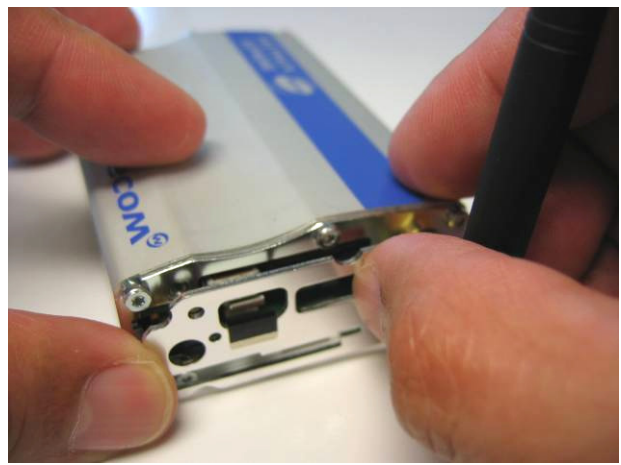
Align the new backplate
