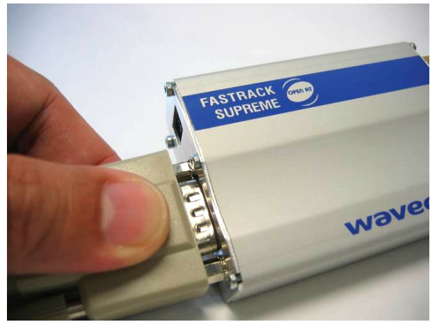
Connect the serial cable D-Sub H.D. to Fastrack Supreme
