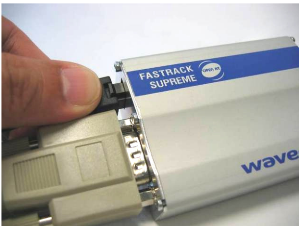
Connect the power adapter cable to Fastrack Supreme
