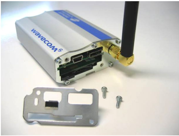
Place the supplied new backplate
