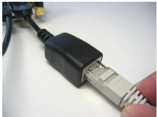
Connect the RJ45 LAN Cable
