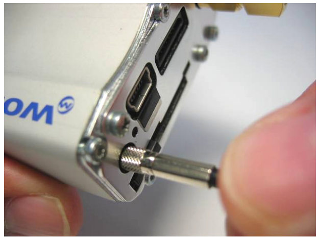
Connect the GPS antenna cable
