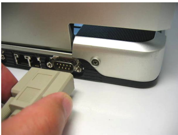
Connect the serial cable other end to PC COM Port
