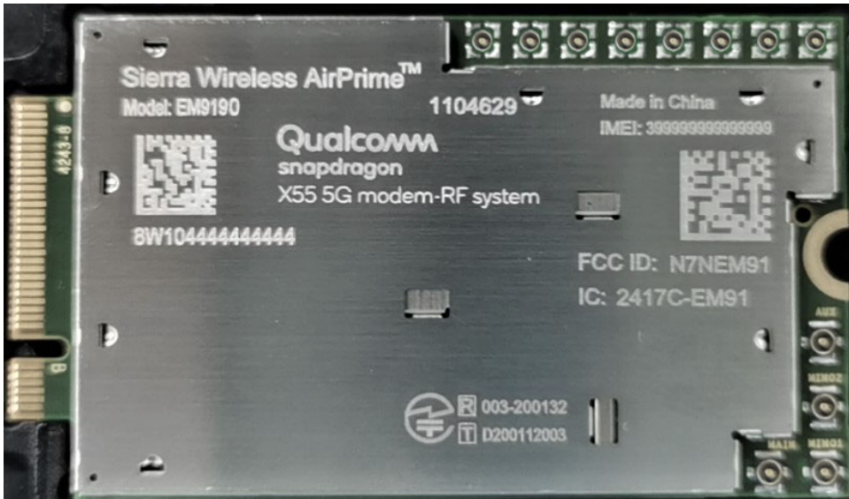
Figure 6-5: Unit Product Marking Example—Laser-etched, Typical Representation (Contents vary by SKU)
