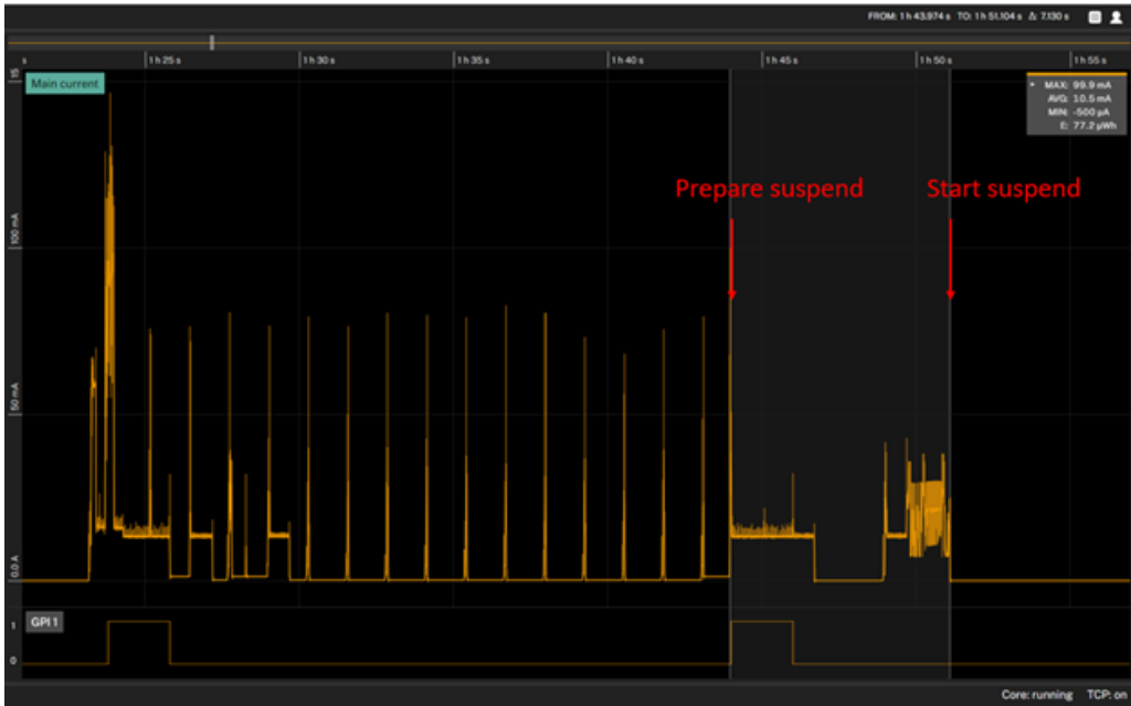
Figure 4-5: HL7810 sleep (modules prepare suspend/hibernation and save memory context to retention memory during preparation)
