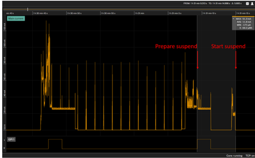
Figure 4-2: HL7800 sleep (modules prepare suspend/hibernation and save memory context to retention memory during preparation)
