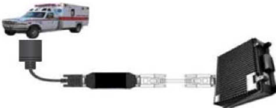
Figure 6-1: Connecting a Scanner Between the oMG and a Heavy Duty Vehicle
