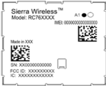
Figure 6-1: Unit Product Marking—Laser-etched, Typical Representation
