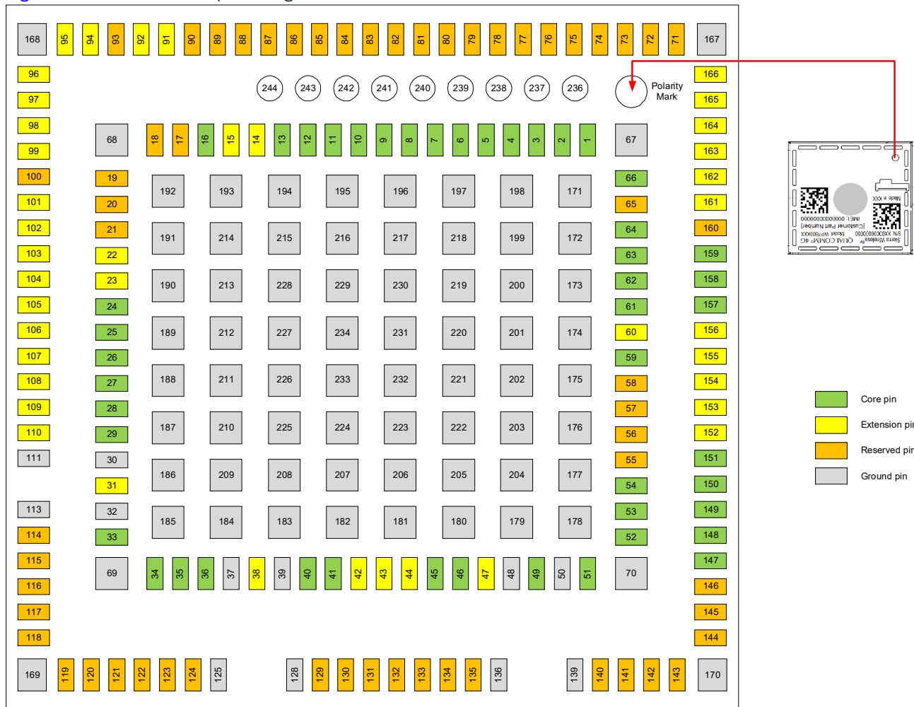
Figure 10-1: Pin Configuration (Top View, Through Module)
