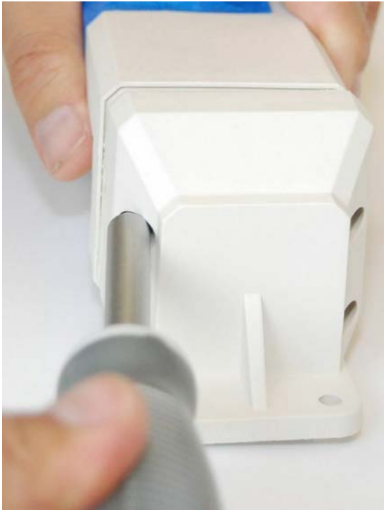
Figure 40 - Removing the Four Screws from the Cap Housing
