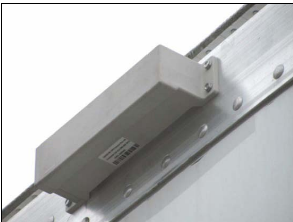
Figure 37 - Chassis mounting with the Device Facing down Nose Mount and Intermodal Container Placement
