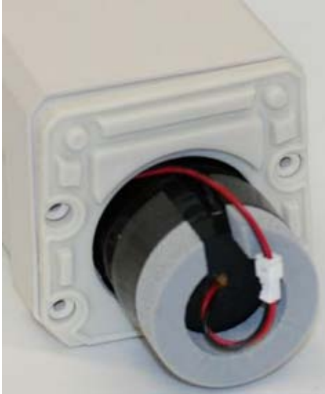
Figure 13 - Replacing the Gasket
