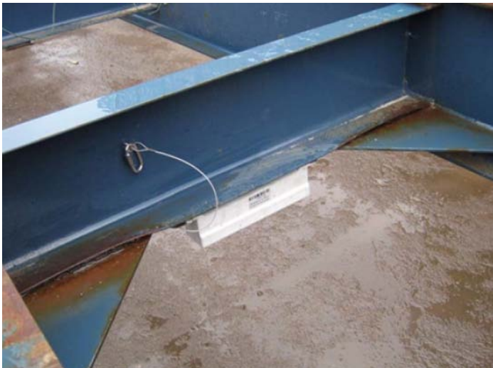
Figure 37 - Chassis mounting with the Device Facing down Nose Mount and Intermodal Container Placement
