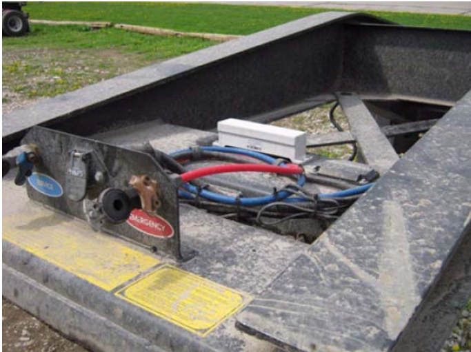
Figure 36 - Chassis Mounting with the Device Facing up
