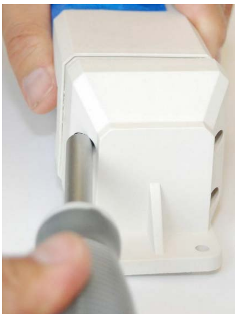
Figure 8 - Removing the Four Screws from the Cap Housing
