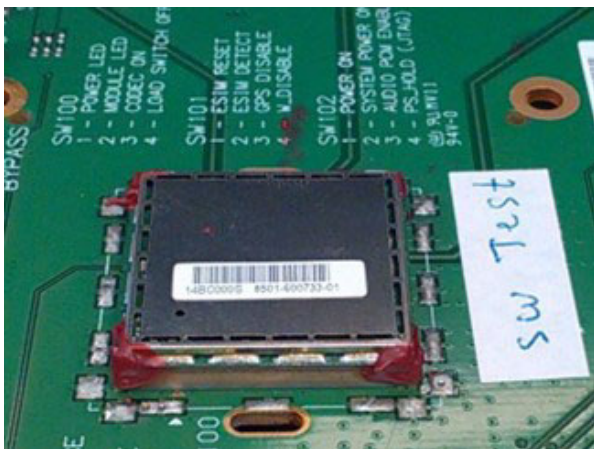
Figure 6-1: Glue deposit on RC module (Example)
