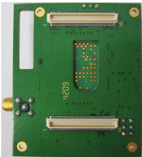
Figure 5. AirPrime WISMO2x8 Socket Board (Bottom View)
