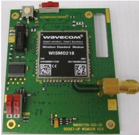
Figure 4. AirPrime WISMO2x8 Socket Board (Top View)
