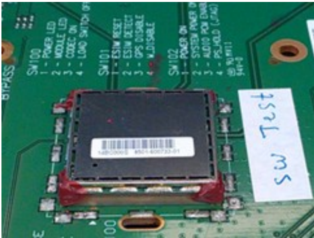
Figure 5-1: Glue deposit on WP module.
