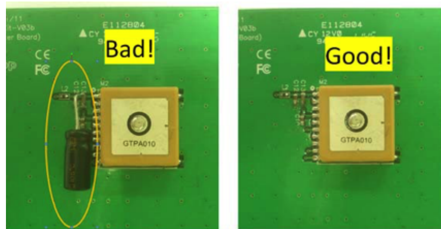
Figure 2-18: First Example of Bad and Good GNSS Module Placement
