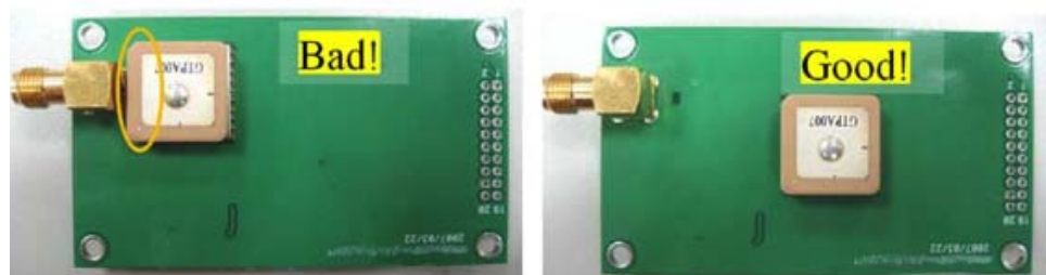
Figure 2-20: Example of bad GPS module placement (Patch Antenna close to a high-profile metal case component) and good placement.
