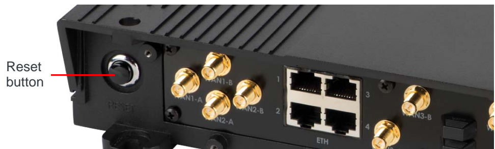
Figure 9-1: Reset Button on Rear Panel of the oMG
