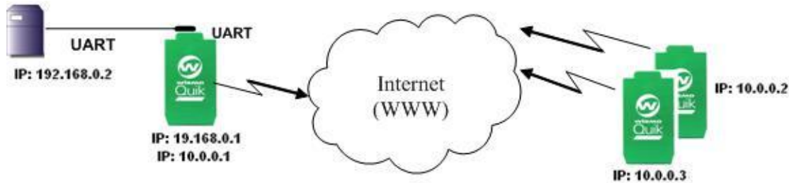
Figure 1. Communication between Four Equipments
