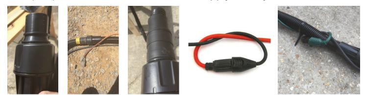
**Step 7:** Connect 90 degree swivel elbow to saw and vacuum hose using 2 in. screw down clamps.
