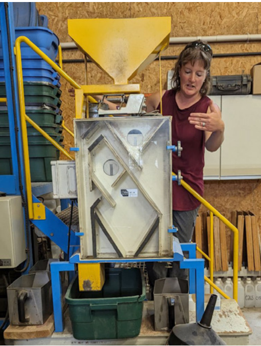
Above: Demonstration of gravity separator at Millson Forestry Service. Photos: Forest Gene Conservation Association
