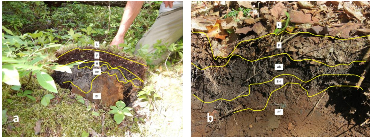
Figure 14: Soil profiles with examples of organic and mineral soil horizons. (adapted from Hazlett et al., 2020) https://www.mdpi.com/2571-8789/4/3/54
