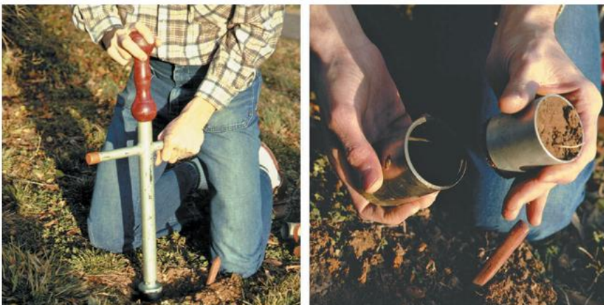
Figure 22: Bulk density sampling with a drop hammer sampler. (Weil and Brady, 2017)
