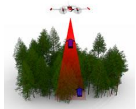
Figure 19. Aerial LiDAR measures the time it takes for a laser to strike an object and return to the source (NRCan 2015).
