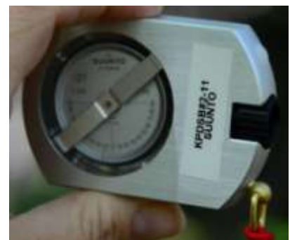
Figure 16. A clinometer is used to measure tree height (Forests Ontario).
