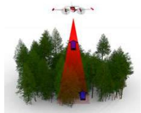
Figure 19. Aerial LiDAR measures the time it takes for a laser to strike an object and return to the source (NRCan 2015).
