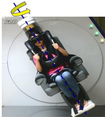
Figure 1: Schematic performance of off-vertical axis rotation test. Subject is seated in a computer-controlled rotary chair. The chair rotates in yaw at a speed of 90 degrees per second while tilted at 30-degree angle to induce motion sickness in the subject.
