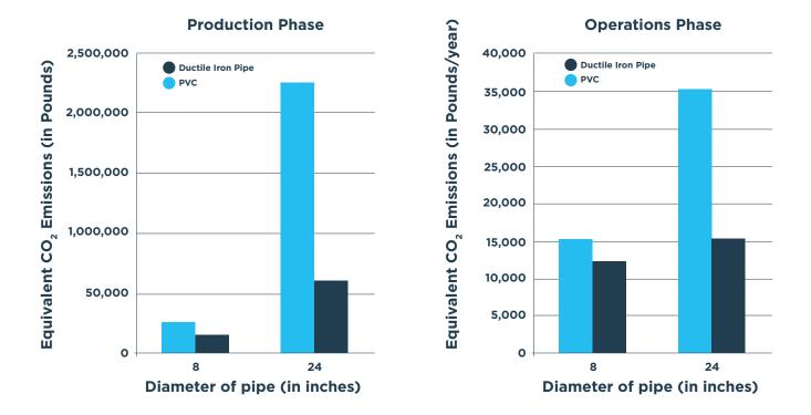
Total equivalent  $\rm CO_2$  emissions assuming 25% pumping during operations phase
