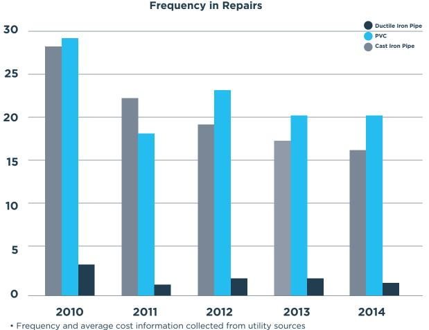
• The cost of individual repair and maintenance is obtained from literature (RSMeans 2015, Haas 2012)
