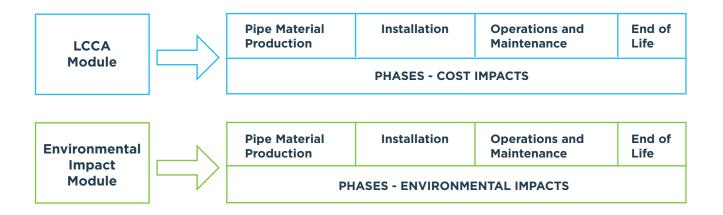
A comprehensive literature search to evaluate a consensus of expected service lives, compilation of cost factors from industry and utilities for purchase and maintenance, and evaluation of the impact of energy use of Ductile Iron Pipe and PVC pipes.
