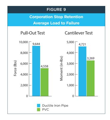
The dramatic difference in values is even more significant because the failures of taps in the Ductile iron pipe tests were failures of the brass corporation stops. No damage was done to the pipe. In each case, failures of the taps in PVC pipe were failures of the pipe wall itself. This distinction is very important to the relative difficulty of repair. For more information, please see our tapping comparison brochure: Tapping Ductile Iron Pipe vs. Polyvinyl Chloride Pipe
