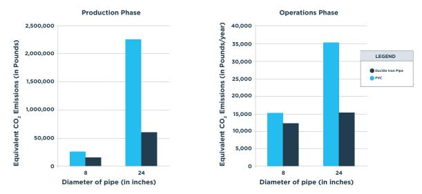
Total equivalent CO<sub>2</sub> emissions assuming 25% pumping during the operations phase
