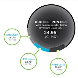
Ductile iron pipe has a larger inside diameter than other pipe materials, and a comparably smooth inner surface.
