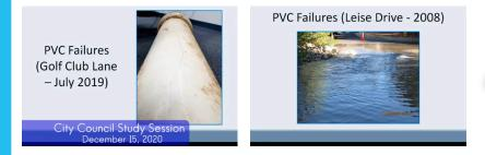
In 1986, a PVC pipe in the city of Prescott exploded/ ruptured injuring two workers. The plastic pipes that we have running under much of Prescott may have been cheaper to initially purchase when past city leaders chose to use them, but they crack more easily, don't last as long, and can actually lose some of their ability to handle pressure at higher temperatures in the soil or even melt if exposed to high temperatures from a fire."
