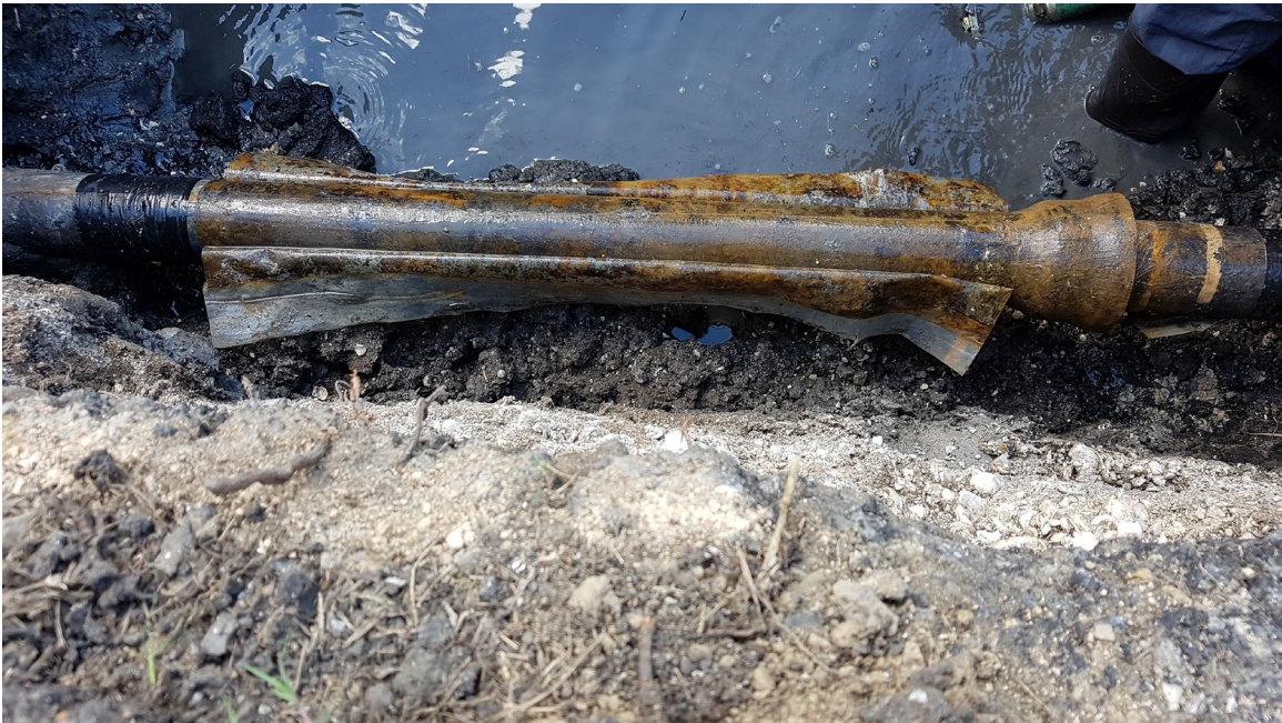
B: Polyethylene sleeving partially removed
