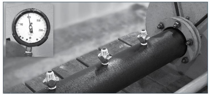
DIPRA's direct tapping tests were conducted on 4-foot Ductile Iron Pipe specimens 6 inches in diameter. Tests involved three 3/4-inch taps on one specimen and three 1-inch taps on the other specimen as shown here. The initial internal water pressure of 70 psi was gradually increased to 1,000 psi (inset photo) in an attempt to cause failure.
