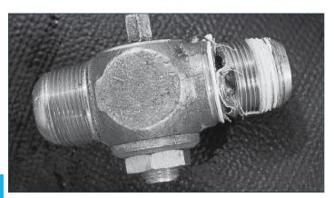
As was the case in the pull-out tests, sufficient cantilever forces damaged the corporation stop, causing the leakage seen in the photo above (top). Damage to the corporation stop is shown above (bottom).
