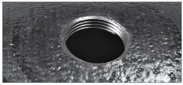
Forces exerted during pull-out tests, when sufficient, resulted in failure of the corporation stop, not the Ductile Iron Pipe or threads. The top photo shows leakage at the plug key of the corporation stop. Ultimate failure occurred to the corporation stop's threaded connection for the service line. The undamaged Ductile Iron Pipe and threads are shown in the photo below.
