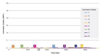
Corrosion rates of all probes under V-Bio® enhanced polyethylene encasement with inhibitor and anti-microbial are at or near zero MPY.
