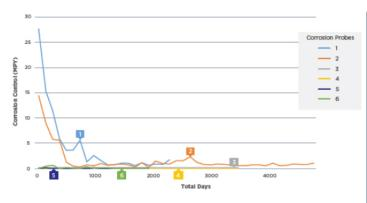
The lower MPY readings of probes inserted under polyethylene encasement was caused by deoxygenation of the aqueous environment trapped underneath the film when the pipe was installed.
