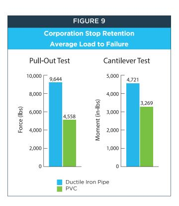
The dramatic difference in values is even more significant because the failures of taps in the Ductile iron pipe tests were failures of the brass corporation stops. No damage was done to the pipe. In each case, failures of the taps in PVC pipe were failures of the pipe wall itself. This distinction is very important to the relative difficulty of repair. For more information, please see our tapping comparison brochure: <u>Tapping</u> <u>Ductile Iron Pipe vs. Polyvinyl Chloride Pipe</u>
