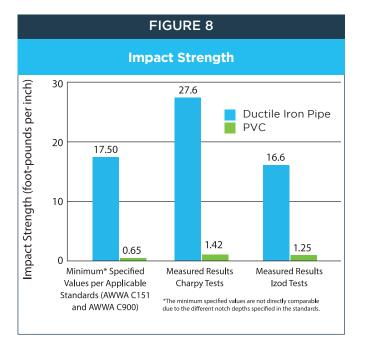
Direct Tapping Ductile Iron Pipe is Easier, less Expensive, Faster—and Less Likely to Damage the Pipe—Than Tapping PVC
