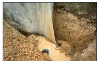
The J-M installation guide provides explicit safety precautions for tapping PVC pipe under pressure. One of those precautions is to "prepare a means of simple and quick exit from the work area in the event of flooding. A sturdy ladder is recommended." With PVC pipe failures such as these, such advice is worthwhile.
