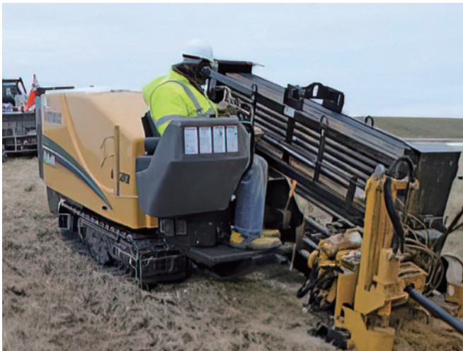
Figure 4: HDD boring machine – courtesy of Trenchless Technology Magazine
