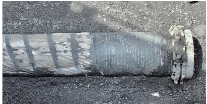
Figure 18: Exposed V-Bio® enhanced polyethylene encasement after HDD installation—Polyethylene encasement uncompromised from installation
