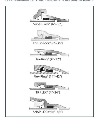
Gripping push-on joint gaskets that utilize stainlesssteel teeth locking segments are not recommended for HDD installations. Joint deflections or relative rotation between two pipe sections during installation with these types of restrained joint gaskets could result in leakage or possible joint separation.
