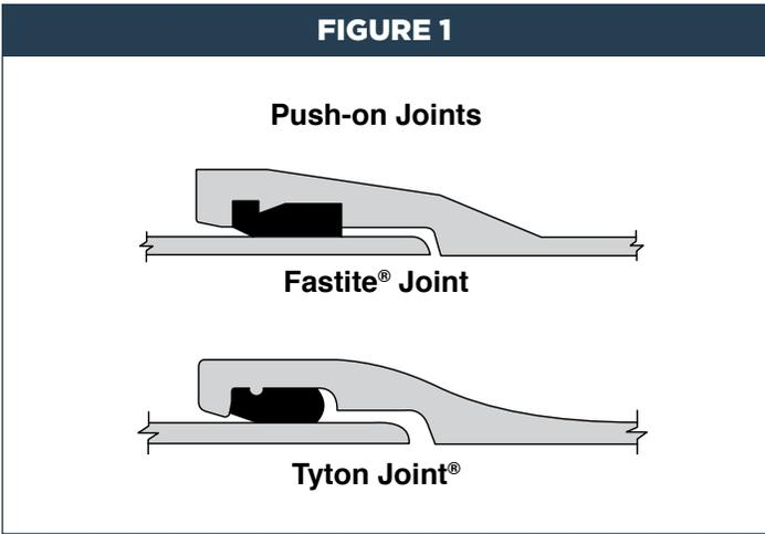
Since standard push-on and mechanical joints are not “restrained,” due consideration should be given to proper design and construction of supports or anchorages to resist thrust forces, dead loads, impact and shock loads, and thermal changes.
