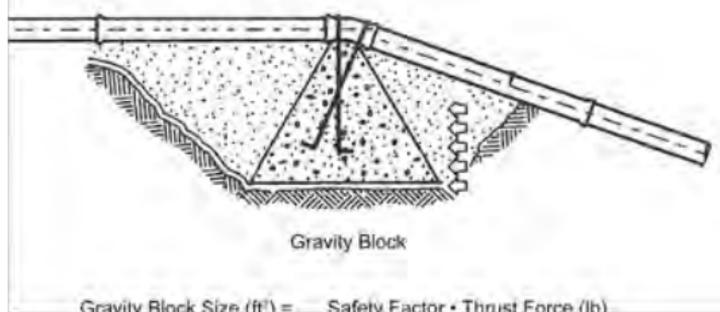
$$\text{Gravity Block Size (ft}^3\text{)} = \frac{\text{Safety Factor} \cdot \text{Thrust Force (lb)}}{\text{Density of Block Material (lb/ft}^3\text{)}}$$
