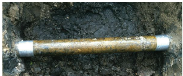
Superficial oxidation of cast iron pipe since 1958
