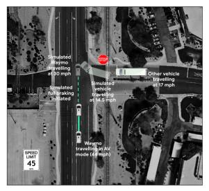
Figure 5. Event D - Simulated Waymo traveling straight with other vehicle failing to stop at a stop sign and not yielding right-of-way to Waymo vehicle
