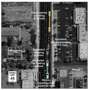
Figure 2. Event A - Simulated head-on collision involving the other vehicle traveling the wrong way
