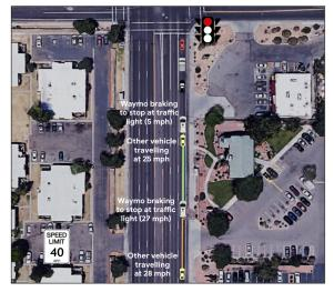
Figure 3. Event B: A rear end collision that resulted in airbag deployment for the vehicle that struck the Waymo vehicle. Sole collision in driverless mode, without a trained operator in the driver's seat.
