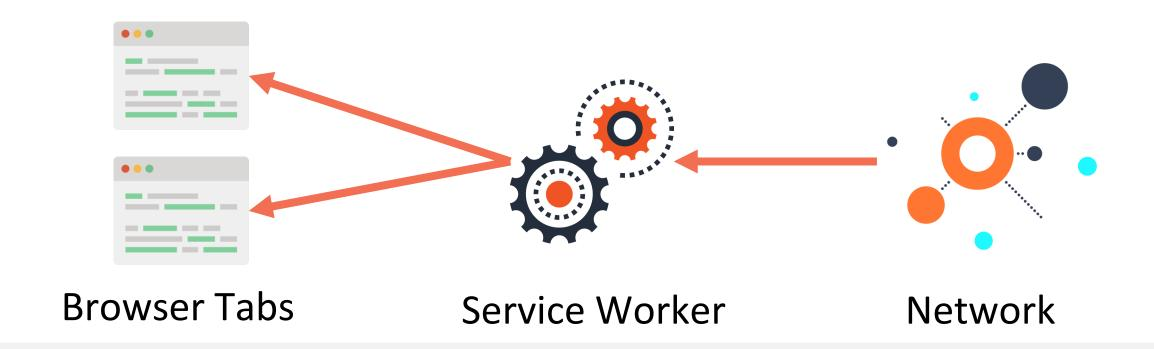
Programmable Network Proxy, running as a separate Background Process, without any DOM Access.
