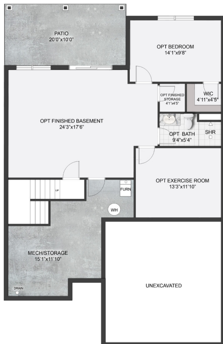
OPT LUXURY REAR WALKOUT FOUNDATION PLAN W/ OPT FINISHED BASEMENT
