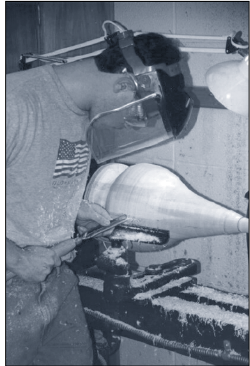
Make sure the tool rest is secure and set close to the stock.
