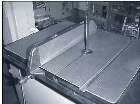
Large portion of exposed blade at point of operation.
