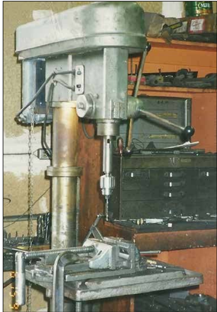
Vertical drill press with vise (to prevent stock from spinning).
