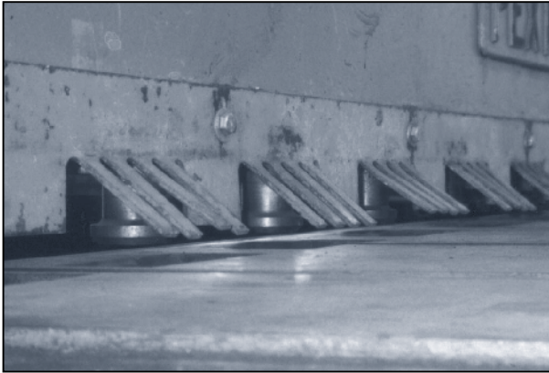
Adjustable barrier-type guarding for the hold-down devices must accommodate stock, not fingers.
