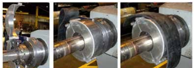
Fabricated quill-mounted guard to enclose cathead.
