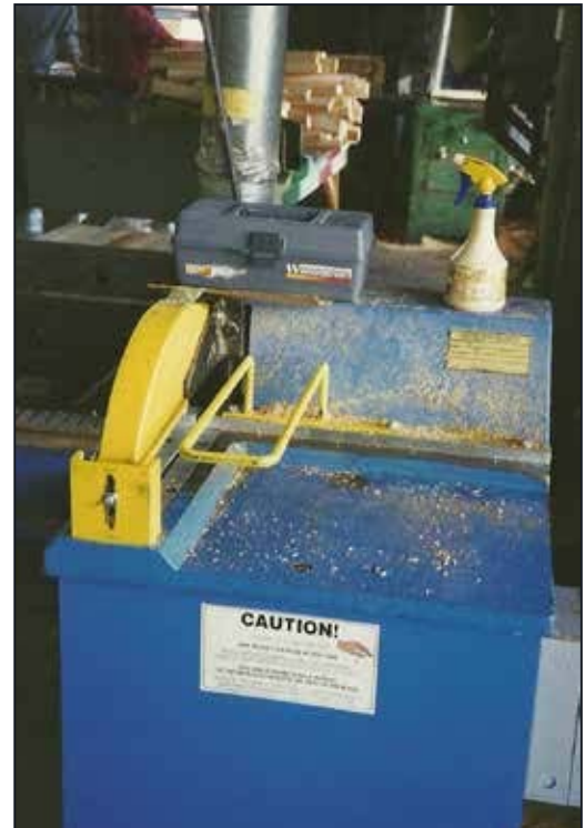
Properly guarded jump saw.
