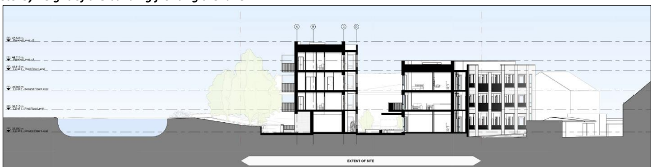
Figure 6: Section through the proposed buildings, showing the four storey height of the canal-front building and the three storey height of the building fronting the lane
