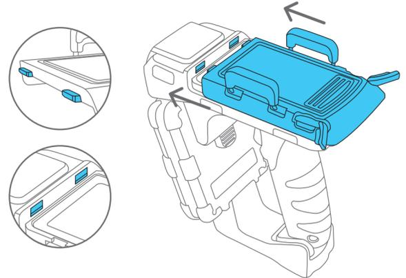
5. Fully rotate to close the metal latches to secure the battery cover in position.
