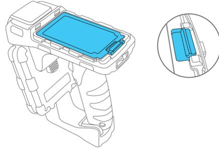
4. Replace the battery cover. Make sure that the locking tabs at the front of the battery cover are fully inserted into the slots.
