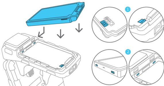
3. The battery should be fully secured by the battery spring-loaded clip as shown.
