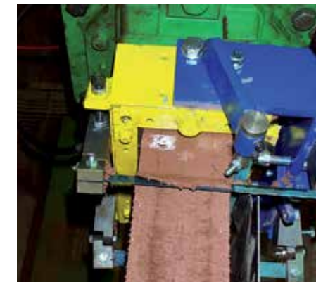
Serrated blades are used to achieve a roughened surface by 'peeling' back the outer surface of the clay.
