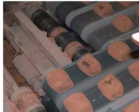
Clots of clay are transported along conveyors to be dropped into the prepared mould boxes.
