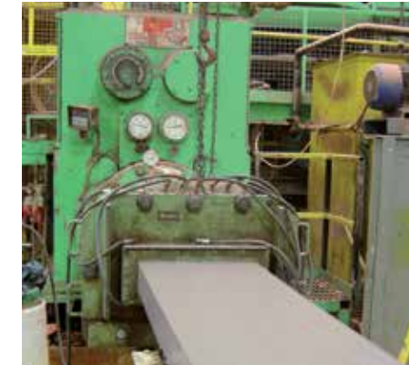
Ibstock's 'Fireborn' product during the extrusion process. A 'die' can be modified to accommodate various size formats.
