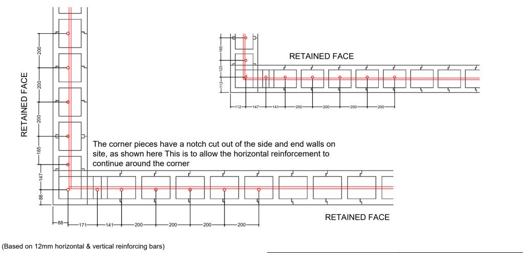
Consideration should be given to the avoidance of creep when setting out the vertical reinforcing bars
