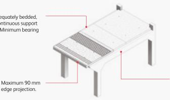
Trestle slab coping stone supports (reinforced concrete support frames) must be adequate to support the coping stone and the requisite imposed loading.
