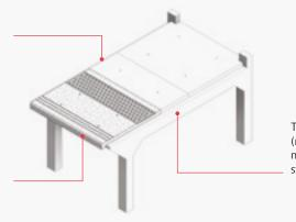
Trestle slab coping stone supports (reinforced concrete support frames) must be adequate to support the coping stone and the requisite imposed loading.
