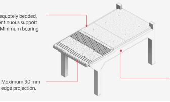
Trestle slab coping stone supports (reinforced concrete support frames) must be adequate to support the coping stone and the requisite imposed loading.
