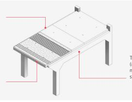
Trestle slab coping stone supports (reinforced concrete support frames) must be adequate to support the coping stone and the requisite imposed loading.
