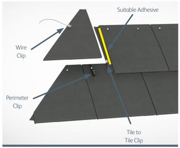
In addition to bonding, perimeter clips or wire clips can also be used to provide a second fixing. When bonding tiles, adhesive should be applied liberally to the full length of the underlock in accordance with the adhesive manufacturer's instructions.
