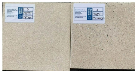
Ibstock Tellings: GRC sample swatches: rcf_002A—with (LH) light blast and (RH) Polished surface treatments
