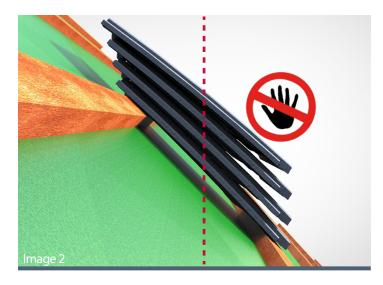
Image 2 shows a side view of the SL8 tile stack. As can be seen from this image, contact with the front edge of the stack must be avoided as it will cause the tiles to become unstable.
