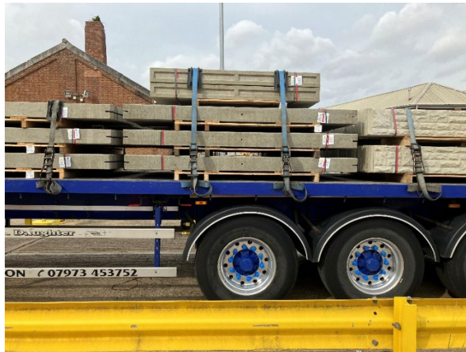
A mixed load with some elements pyramid stacked, straps a placed close to the bearers to prevent damage
