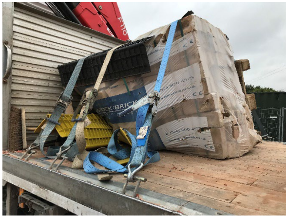
Incorrectly loaded bricks moved during braking
