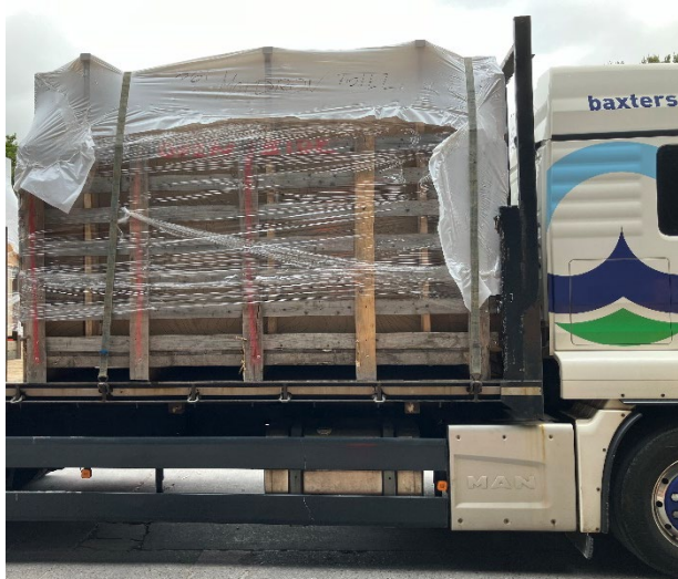
Futures load packed into a crate, wrapped and secured with two straps
