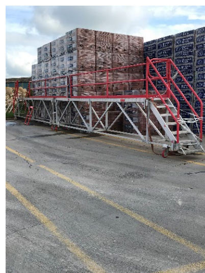
Movable access gantry
