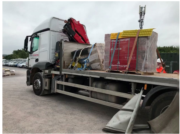
Incorrectly loaded bricks moved during braking
