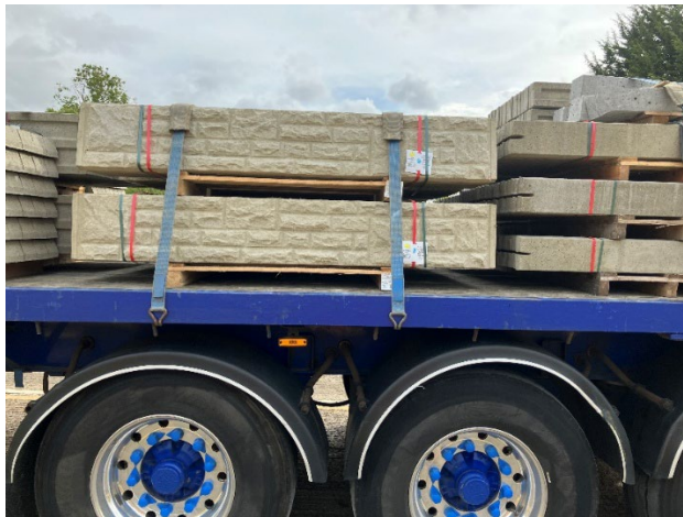
Product over 600 mm wide secured with two straps close to the bearers
